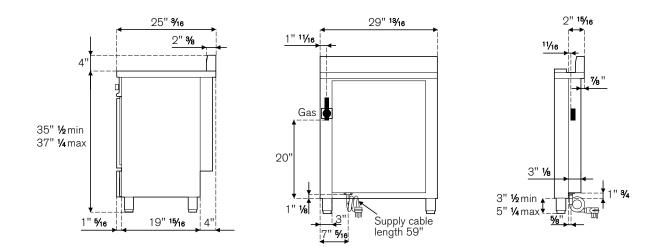
Bertazzoni recommends to operate the appliance after it has been installed in a cabinet. The kitchen cabinets shall be made of materials capable of withstanding temperatures at least 117°F (65°C) above room temperature in order to avoid possible damage to the cabinets during oven usage. For further installation instructions refer to the installation manual.
